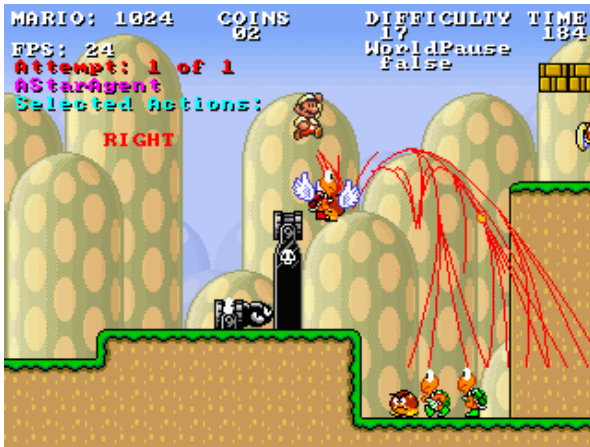
Fig. 5. Visualization of the future paths considered by the A* controller. Each red line shows a possible future trajectory for Mario, taking the dynamic nature of the world into account.
