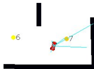
Fig. 4. Sensor setup of the further evolved general controller analysed in table V. Only three sensors seem to be long enough to of any use, and all of those point to the right or front-right. The asymmetry and "waste" is somewhat surprising, as the controller performs well on all the first six tracks (but it does do slightly better on clockwise than on anti-clockwise tracks).
