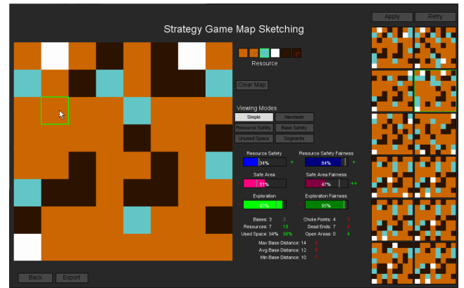
Figure 1: The Sentient Sketchbook tool during a design session. To the left is the sketch editor, far to the right are the automatically generated map suggestions; between these elements is the tile palette, the map display menu and an overview of map’s fitness dimensions and metrics.
